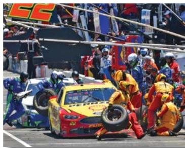
Race car tires are filled with **nitrogen gas** instead of air. Nitrogen is a drier gas and gives the race team more control over how fast the air pressure builds in the tires.
